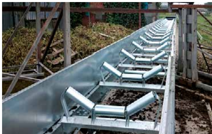
Detailed view of triple rollers
